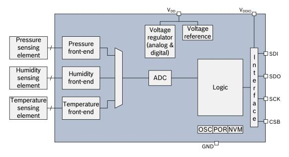
Figure 2: Block diagram of BME280
