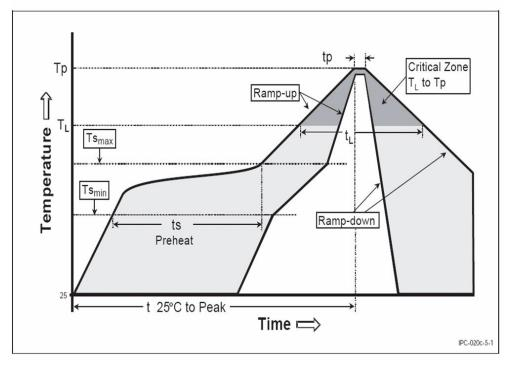
Figure 22: Soldering profile
