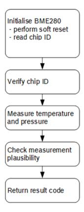
Figure 25: Self-test flow chart
