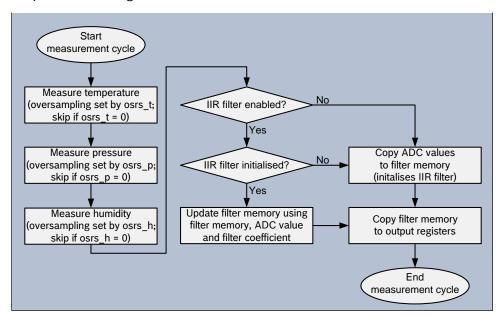
Figure 6: BME280 measurement cycle
