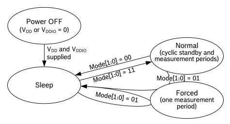
Figure 3: Sensor mode transition diagram
