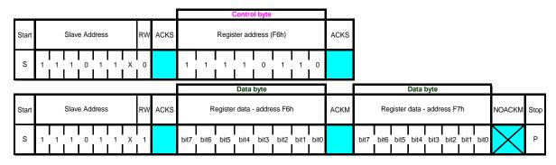
Figure 10: I2C multiple byte read
