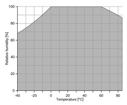
Figure 1: humidity sensor operating range
