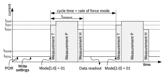
Figure 4: Forced mode timing diagram
