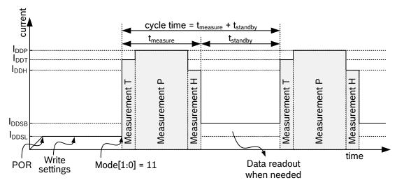
Figure 5: Normal mode timing diagram
