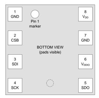
Figure 16: Pin-out top and bottom view
