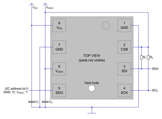
Figure 17: I<sup>2</sup>C connection diagram
