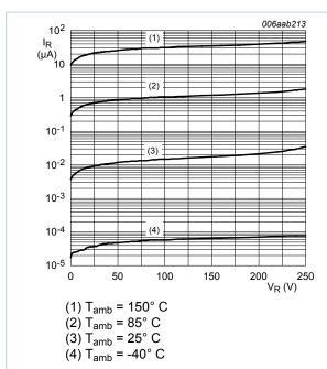
Fig. 6. Reverse current as a function of reverse voltage; typical values
