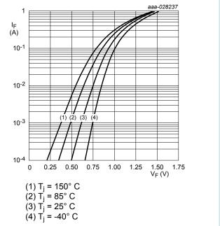
Fig. 5. Forward current as a function of forward voltage; typical values; (logarithmic scale)
