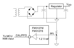
The voltage on the PFI input pin is compared to an onboard 1.2 V reference. When the PFI input voltage drops below this threshold, the comparator will drive the CAL/PFO pin to a ILOW state. The comparator has 100 mV (max) of hysteresis to reduce noise sensitivity, only for a rising PFI signal. For a falling PFI edge, there is no hysteresis.
