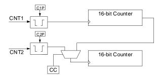
The control bits for event counting are located in register 0Ch. Counter 1 Polarity is bit C1P, bit 0; Counter 2 Polarity is C2P, bit 1; the Cascade Control is CC, bit 2; and the Read Counter bit is RC, bit 3.
