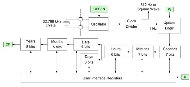
Figure 7. Real-time Clock Core Block Diagram
