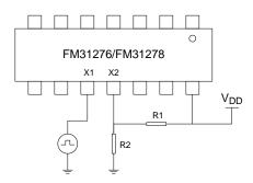
In the example, R1 and R2 are chosen such that the X2 voltage is centered around the X1 oscillator drive levels. If you wish to avoid the DC current, you may choose to drive X1 with an external clock and X2 with an inverted clock using a CMOS inverter.
