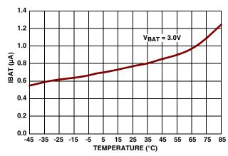
FIGURE 4. I<sub>BAT</sub> vs TEMPERATURE
