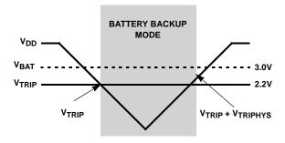
FIGURE 10. BATTERY SWITCHOVER WHEN VBAT > VTRIP
