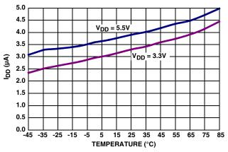
FIGURE 3. I<sub>DD3</sub> vs TEMPERATURE
