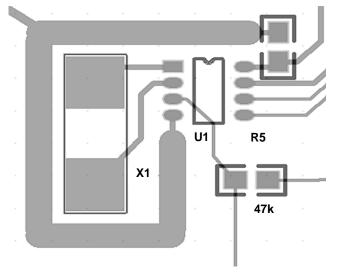
FIGURE 23. SUGGESTED LAYOUT FOR INTERSIL RTC IN SO-8
