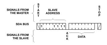
FIGURE 19. CURRENT ADDRESS READ SEQUENCE
