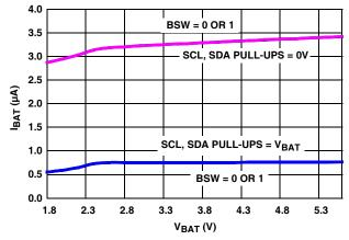
FIGURE 1.  $I_{BAT}$  vs  $V_{BAT}$ , SBIB = 0
