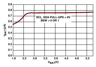
FIGURE 2.  $I_{BAT}$  vs  $V_{BAT}$ , SBIB = 1
