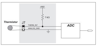
Figure B-6. RCM3700 Prototyping Board Thermistor Input
