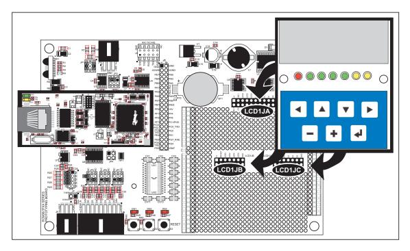
Figure C-8. Install LCD/Keypad Module on RCM3700 Prototyping Board
