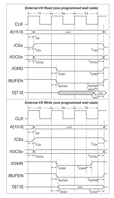
Figure A-4 shows a typical timing diagram for the Rabbit 3000 microprocessor external I/O read and write cycles.
