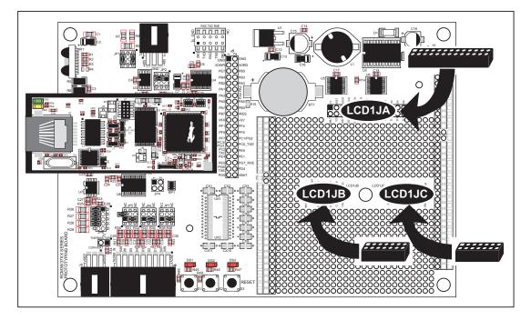
Figure C-7. Solder Connectors to RCM3700 Prototyping Board
