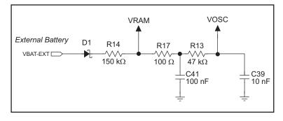
Figure D-2. RCM3700 Backup Battery Circuit
