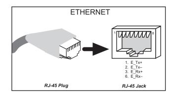
Figure 8. RJ-45 Ethernet Port Pinout
