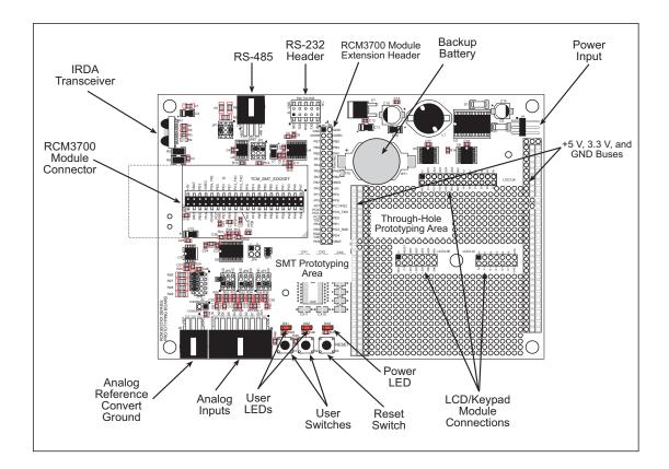
Figure B-1. RCM3700 Prototyping Board
