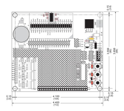
Figure B-12. RCM3720 Prototyping Board Dimensions
