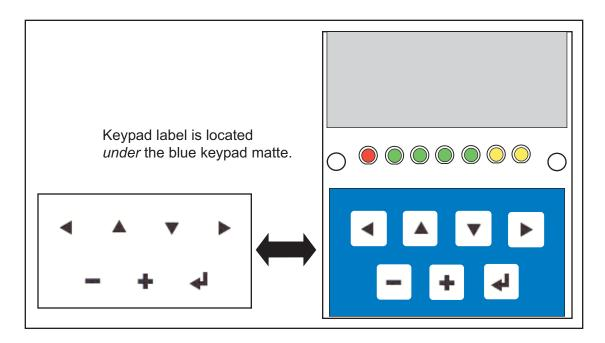
Figure C-5. Removing and Inserting Keypad Label
