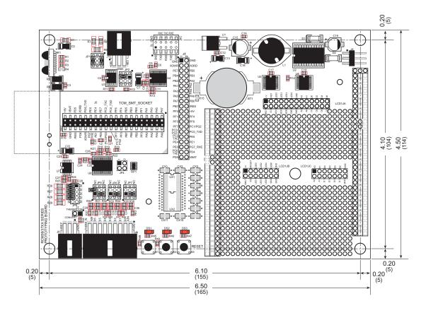
Figure B-2. RCM3700 Prototyping Board Dimensions
