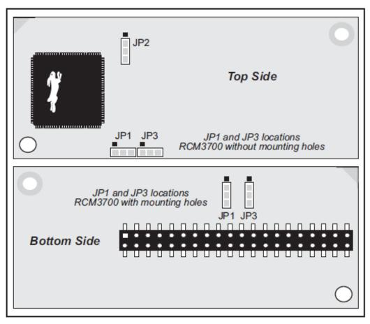
Figure A-6. Location of RCM3700 Configurable Positions
