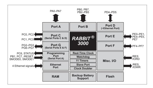
Figure 6 shows the use of the Rabbit 3000 microprocessor ports in the RCM3700 modules.
