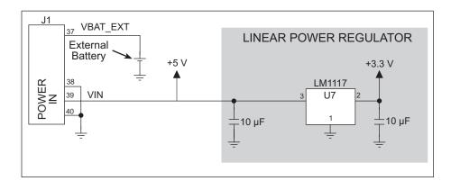
Figure D-1. RCM3700 Power Supply
