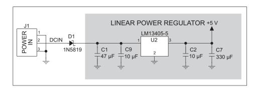
Figure B-13. RCM3720 Prototyping Board Power Supply
