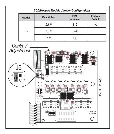
Figure C-3. LCD/Keypad Module Voltage Settings
