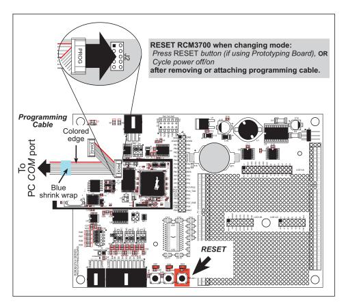
Figure 9. Switching Between Program Mode and Run Mode
