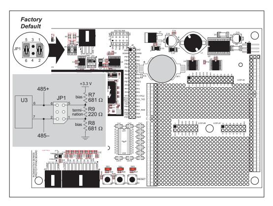
Figure B-9. RS-485 Termination and Bias Resistors
