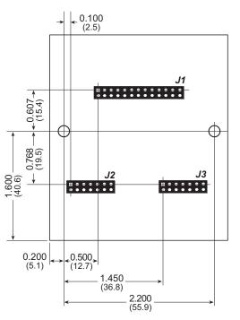
Figure C-2. User Board Footprint for LCD/Keypad Module
