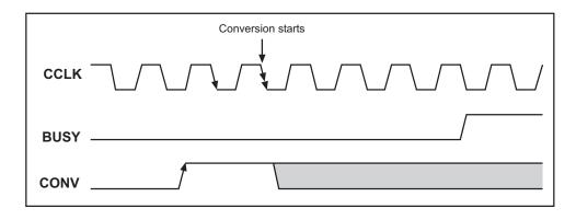
Figure B-7. Timing Diagram for Conversion Start Using CONVERT Pin
