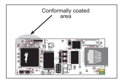
Figure A-5. RCM3700 Areas Receiving Conformal Coating
