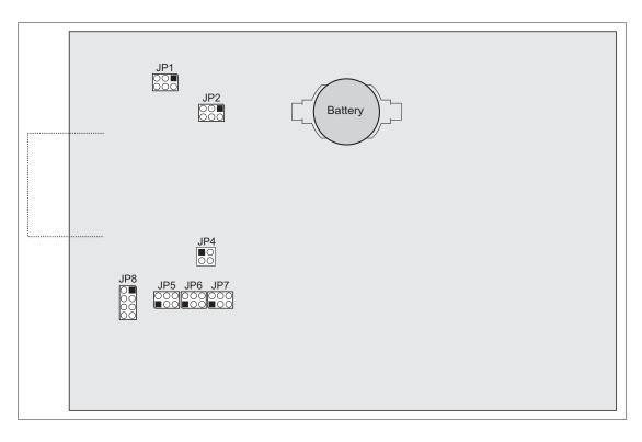
Figure B-10. Location of RCM3700 Prototyping Board Configurable Positions
