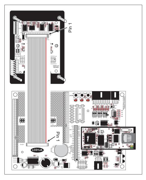
Figure C-11. Connecting LCD/Keypad Module to RCM3700 Prototyping Board
