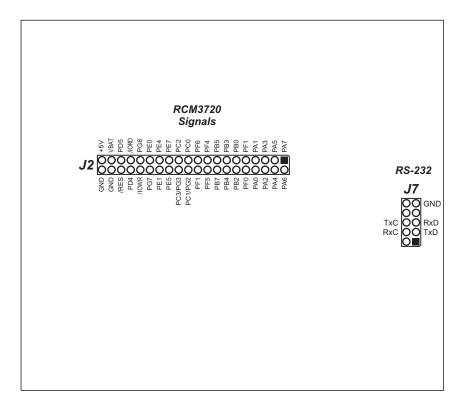
Figure B-14. RCM3720 Prototyping Board Pinout
