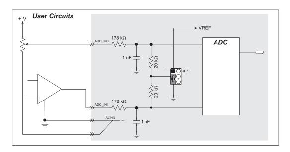
Figure B-5. A/D Converter Inputs
