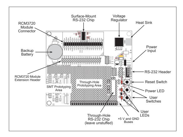
Figure B-11. RCM3720 Prototyping Board
