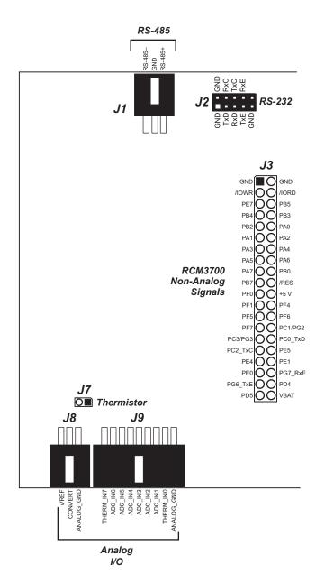
Figure B-4. RCM3700 Prototyping Board Pinout
