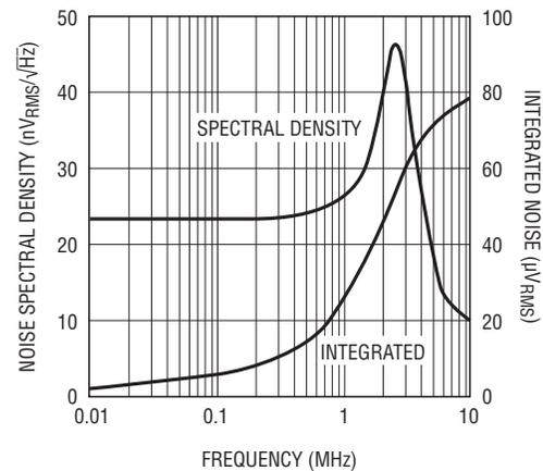
Figure 7. Input Referred Noise, Gain = 1
