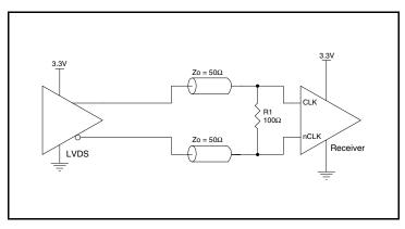
Figure 2E. CLK/nCLK Input Driven by a 3.3V LVDS Driver
