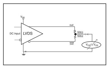
**Differential Output Voltage Setup**
