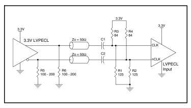
Figure 2D. CLK/nCLK Input Driven by a 3.3V LVPECL Driver with AC Couple
