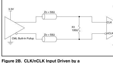
Figure 2B. CLK/nCLK Input Driven by a 3Built-In Pullup CML Driver
