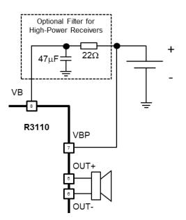
Figure 3. Typical High–Power Filter
